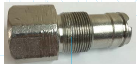
Damage to threads on SDX III Nozzle
