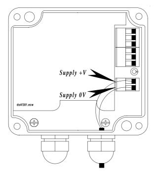
The DS10CC requires a DC power supply of between 12V and 24V 80mA. Referring to the figure to the left of this text, the supply cable should be passed through a convenient cable gland and should be connected as shown. The supply connections are identified on the Printed Circuit Board.
