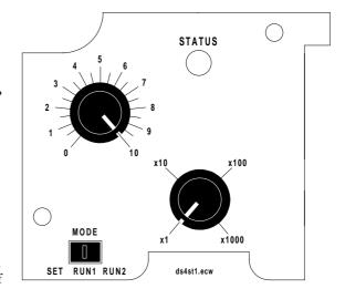
After an initial delay of approximately 1 second, the STATUS LED will illuminate. The colour of the LED is not important at this point.
