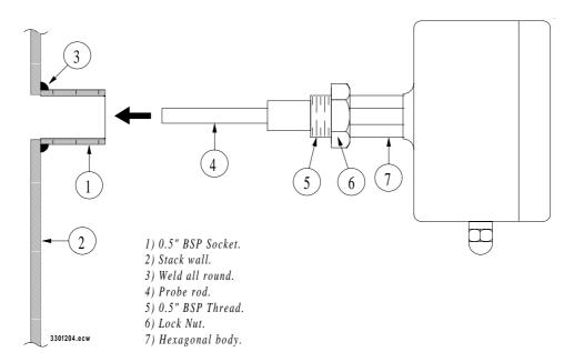
Referring to the diagram above, the sensor is mounted to the stack in the following way;
