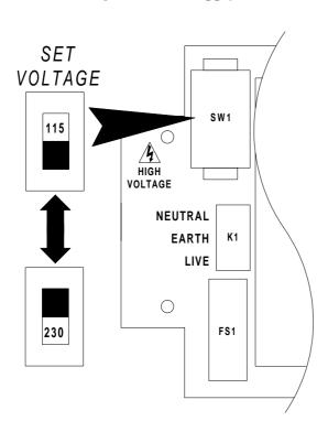
The Dustsense PSU requires a mains power supply of either 115V or 230V @ 50/60Hz. Remove the PSU cover by unscrewing the four pozi-head screws in the deeply recessed holes on the underside of the unit. Referring to the figure to the left of this text, the supply cable should be passed through the cable entry grommet supplied and should be connected to K1 as shown. Mains cable with a 3A rating will be adequate. This
