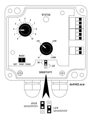
If during STEP 2 of the set-up procedure it is not possible to make the 'status' LED change colour from red to green, then it is recommended that the sensitivity be reduced in the sensor unit.
