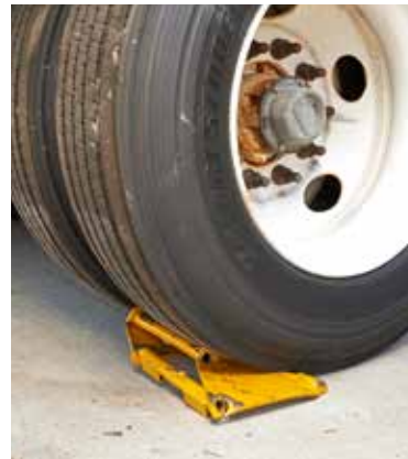
Wheel chock crushed by a truck at the loading dock
