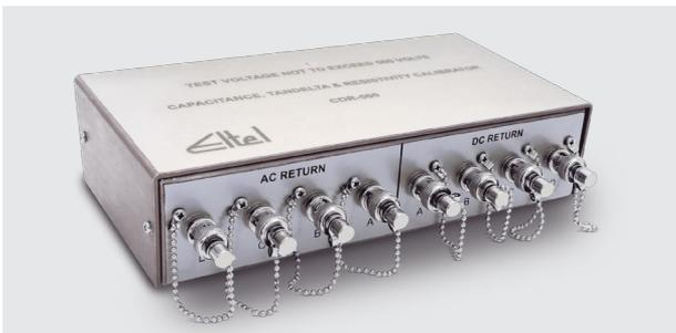
This calibration box is used to routinely check and inspect the Test Set. The Calibrator offers one Capacitance, three Tan Delta & four Resistivity values. The maximum operating voltage is 500V AC or DC.
