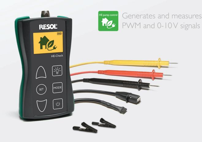
The HE-Check takes over where conventional tools fail — at the question whether a malfunction is caused by a pump fault or the controller signal. With the HE-Check, the function of the pump and the signals of the controller can be checked quickly and easily. The testing device measures and generates 0-10V pump control signals as well as PWM signals in a frequency range from 40 up to 2000 Hz.
