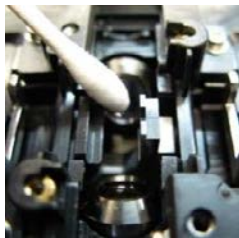
Detachable V-groove and Easy Cleaning
