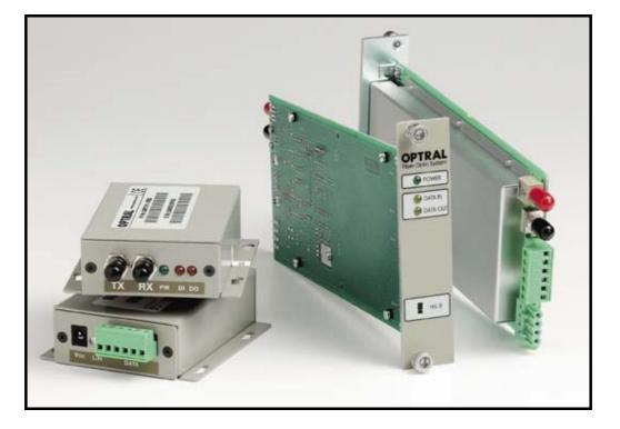
The OPTRAL Series DS5 allows the transmission and reception of RS232, RS422 and RS485 data signals over singlemode optical fibre. The basic system consists of two transceiver and two fibre optics for each communication channel with speeds up to 115 Kbs. The communication protocol: RS232, RS422, RS485-2H (2 Wires Half Duplex) and RS485 4H (4 Wires Full Duplex), can be selected by a switch.
