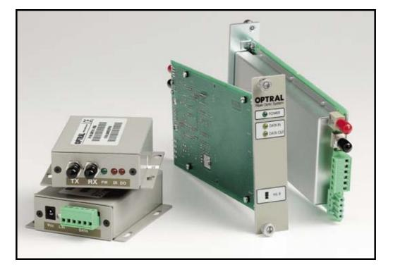
The OPTRAL Series DM5 allows the transmission and reception of RS232, RS422 and RS485 data signals over multimode optical fibre. The basic system consists of two transceiver and two fibre optics for each communication channel with speeds up to 115 Kbs. The communication protocol: RS232, RS422, RS485-2H (2 Wires Half Duplex) and RS485 4H (4 Wires Full Duplex), can be selected by a switch.
