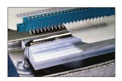
Flow wells match the lead pattern and determine the size, shape and direction of solder flow. Air-Vac maintains an assortment of standard flow wells and cleaning hoods. Flow wells can be made up to 15" long and have multiple process sites.
