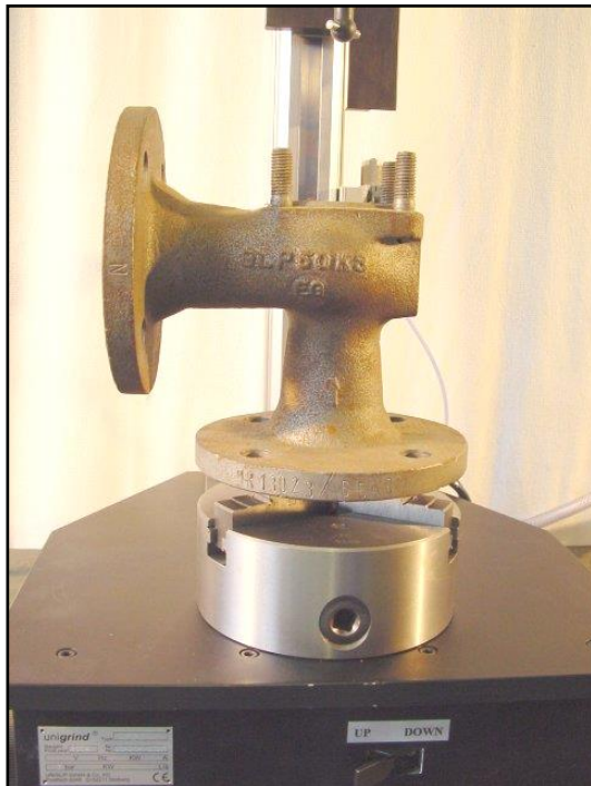
Clamping the valve flange with Inside Jaws at the flange bore
