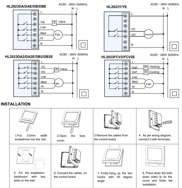
Note: Be sure to connect all the wires as per the wiring diagrams and keep it away from water, mud and other material so as to prevent the unit being spoiled!
