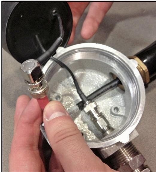
Figure 20: Female Plug to Male BNC Head
