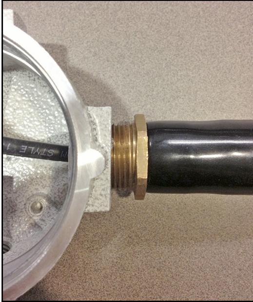
Figure 17: Torquing the Cable Gland
