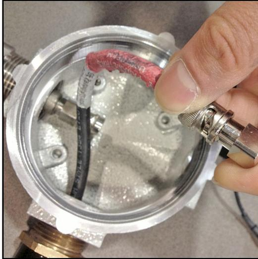
Figure 19: Connecting BNC Plug to the Cable
