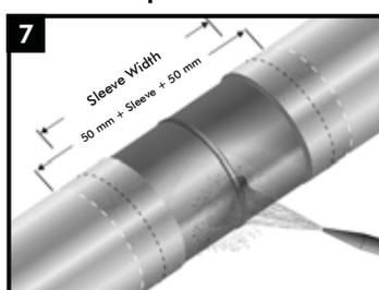
Ensure that the pipe is dry before cleaning. Prepare the steel joint area using the Surface Preparation and Pre-Heat Chart as a guideline. Lightly abrade the pipe coating adjacent to the cutback area to a distance of 50mm (2") beyond each end of the sleeve width.
