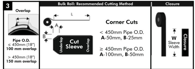
As a guideline, cut the required lengths of Sleeve material (L) and Closure material (W) from the bulk roll as follows
