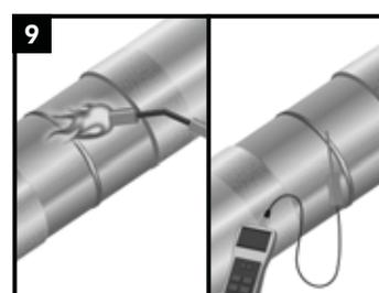
Pre-heat the joint area to the minimum required temperature (see Surface Preparation & Pre-Heat Chart). Using a temperature measuring device, ensure that the correct temperature is reached on the steel and at least 50mm (2") on each side of the sleeve.
