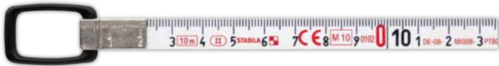
ARCHITECT: White-painted steel measuring blade with cm/mm scale. The o-point is at the start of the tape clasp. Accuracy class II
