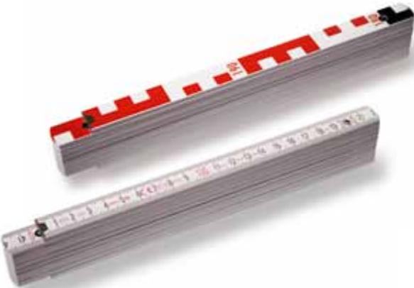
2 m long geo-folding rule – long-distance visible scale with 'E' gradations on one side and classic metric scale on the other.
