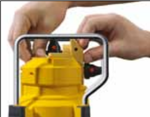
Changing from horizontal to vertical position: the complete prism unit is swivelled precisely by 90° in the guide channel.
