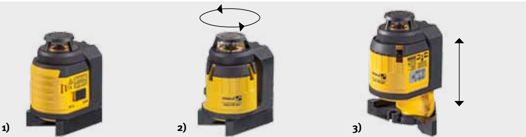
1) Park position. 2) Housing can pivot 360° inside the U-shaped housing. 3) The height of the laser can be adjusted thanks to the extendable foot. The bearing surface enables the laser to be positioned on elements such as U-profiles.
