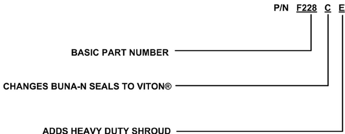
P/N Example: F228CE – Basic F228 coupler is equipped with optional Viton® seals and heavy duty coupler.
