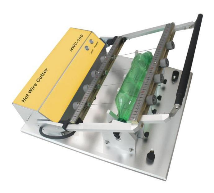
**Test Item: Sectional Cutting for weight analysis**
