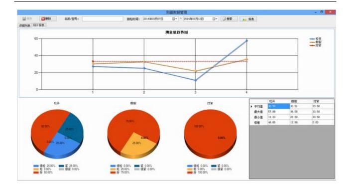
A special software dedicated to reading up to 10000 points / measure with special analog card connected to the torquemeter.
