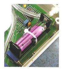
5. Pull out the measuring cell from its socket as shown here. Replace with the new cell. Check that the cell is fully plugged in and the black O ring is correctly positioned
