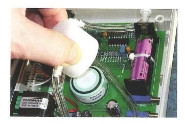
4. Remove and replace the internal battery.
