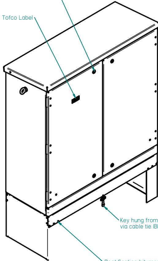
Key hung from root section via cable tie (BK-KEY/R)
