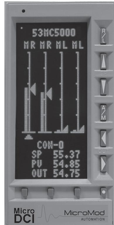
The 53MC5000 is a multiloop, multifunction Process Control Station designed to perform any process application, from simple PID to the most complex control strategy. It combines DCS-style control algorithms with the discrete I/O handling and sequence control of a PLC in one compact package. The high-visibility dot matrix display is available in normal and high-resolution format and supports customized graphic screens and trending in addition to standard operating displays.
