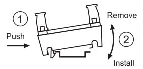
Figure 4.1: DIN Rail Installation and Removal
