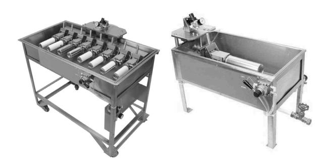
**Test Item: Leak Test for Aerosol Cans**
