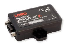
**3DM-GX5-45** – miniature, high-performance, industrial-grade all-in-one navigation solution with integrated multi-constellation GNSS, high noise immunity, and exceptional performance
