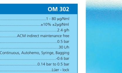
Concentration range Accuracy ..... .....±10% ±2µg/Nml Production rate... Measurement system......ACM indirect maintenance free Continuous flow Operation capability ......Continuous, Autohemo, Syringe, Bagging Vacuum pressure ..... -0.6 bar Syringe automatic pressure control ......0.14 bar to 0.5 bar Ozone output fitting......Lüer - lock Electric supply Oxygen supply... Weight ..... .....16 Kg
