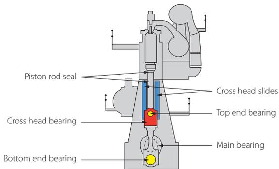
AREAS OF FAILURE – 4 STROKE ENGINE
