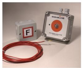
All the controllers are self setting, this avoids any lengthy setting up and calibration process. The controller will react to any significant increase in temperature by detecting the associated change in the cable's resistance.
