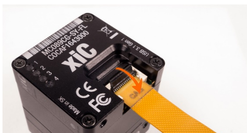
figure 3-40, MC FPC insert procedure option -FL
