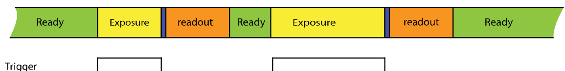
figure 4-7, Exposure defined by trigger pulse length
