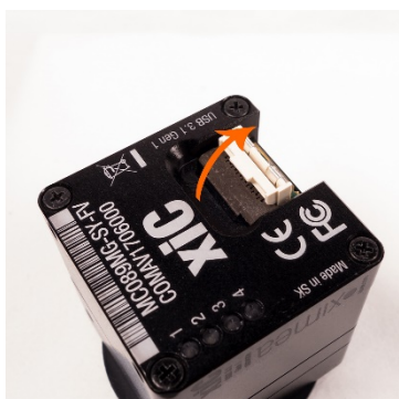
figure 3-41, MC FPC detach procedure option -FL
