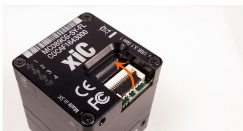
figure 3-39, MC FPC cable CBL-USB3FLEX-xxx ends
