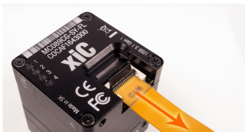
figure 3-41, MC FPC detach procedure option -FL
