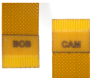
figure 3-38, MC FPC cable CBL-MQ-FL-xxx laser marking
