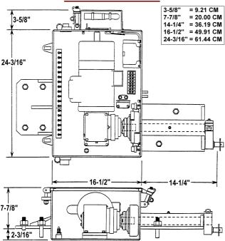
\* Right-hand machine dimensions shown. Same relative dimensions for left-hand machine. Refer to service manual SM-6455 for additional diagrams.
