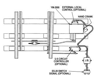
Right-hand machine lauout shown. Same relative placement of equipment for left-hand machine. Refer to service manual SM-6455 for additional diagrams.
