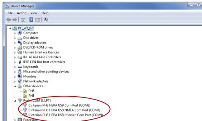
Open a standard terminal program like *PuTTY* (<http://www.putty.org/>). Enter the *COM* port number from the *Cinterion PH8 HSPA USB Com Port* as *Serial line* and change *Parity* and *Flow control* to *None*. Open the *PuTTY* command window.
