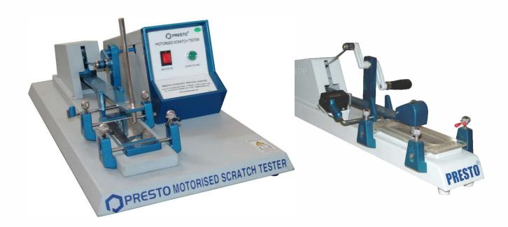
Scratch Hardness Tester - Motorised / Hand Operated
