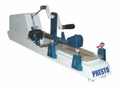
It is a suitable apparatus for carrying out the tests relating to resistance to scratch under a specified load Test are conducted either on a go/no go basic by testing at a single specified load on the needle or by increasing loads to determine the minimum load at which the coating is penetrated.
