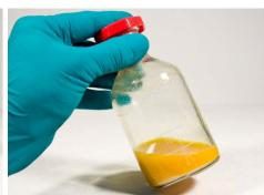
For boiler under 30 bar take a 50 ml water sample in the stoppered bottle provided.
