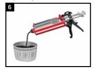
To dispense, unscrew the cap, remove the two small plugs in each side of the cartridge and replace cap. Squeeze the trigger of the cartridge dispenser and dispense a desired amount of material into a mixing cup. The cartridge dispenser will automatically dispense the correct ratio of base and cure.
