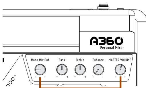
Master Volume must be up to feed the Mono Mix output.
