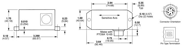
Model AlLSOC: Connector Termination Dimensions inch (mm), approx. values
