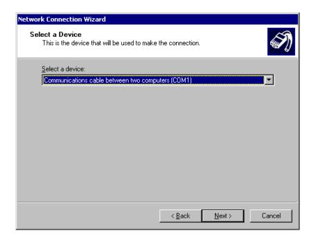
The created "connection cable" has to be selected as device. In the following dialogues, the availability and the name of the connection has to be set. These inputs are optional.
