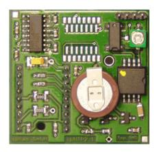
With this GPS / DCF77 Module, the ipNTP with DCF77- or GPS-Antenna is the subject of the description.
