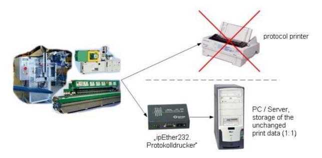
Replace serial/parallel printers and transmit the captured print data via the Ethernet to a central server (on which the capture software is installed).
