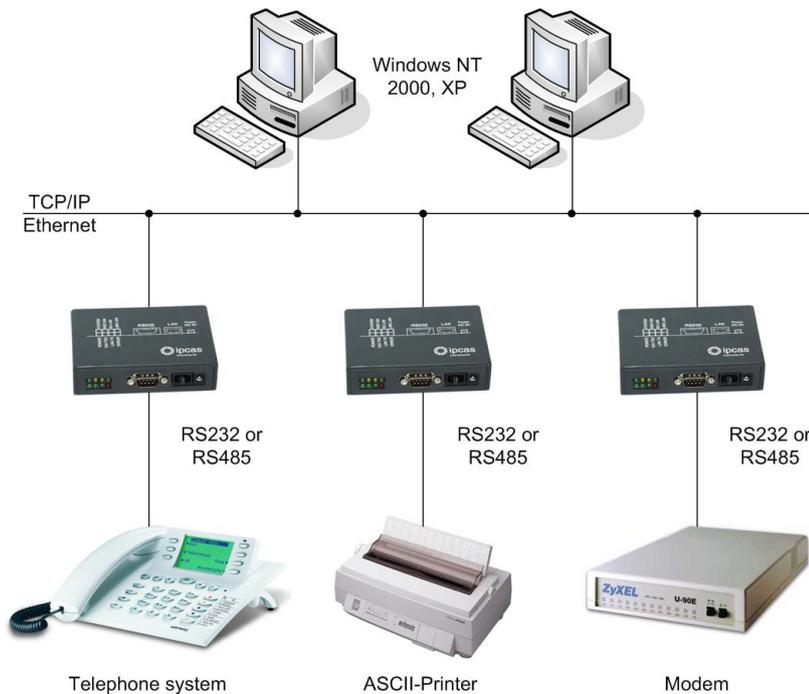
The ipEther232 is characterised by its compact design, its simple integration and the various operational areas. The operational are the automation technology and the building control systems e.g.: CNC machines, testing sets, measuring instruments, telephone systems, modems, serial printers, serial displays and cash plants.
