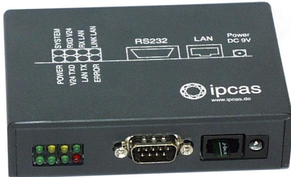
The serial Ethernet converter ipEther232 makes possible controlling of for devices with RS232 or RS485 interface over the Ethernet, by means of a virtual COM Port. This behaves locally like a normal COM Port (e.g.: Com 5).
